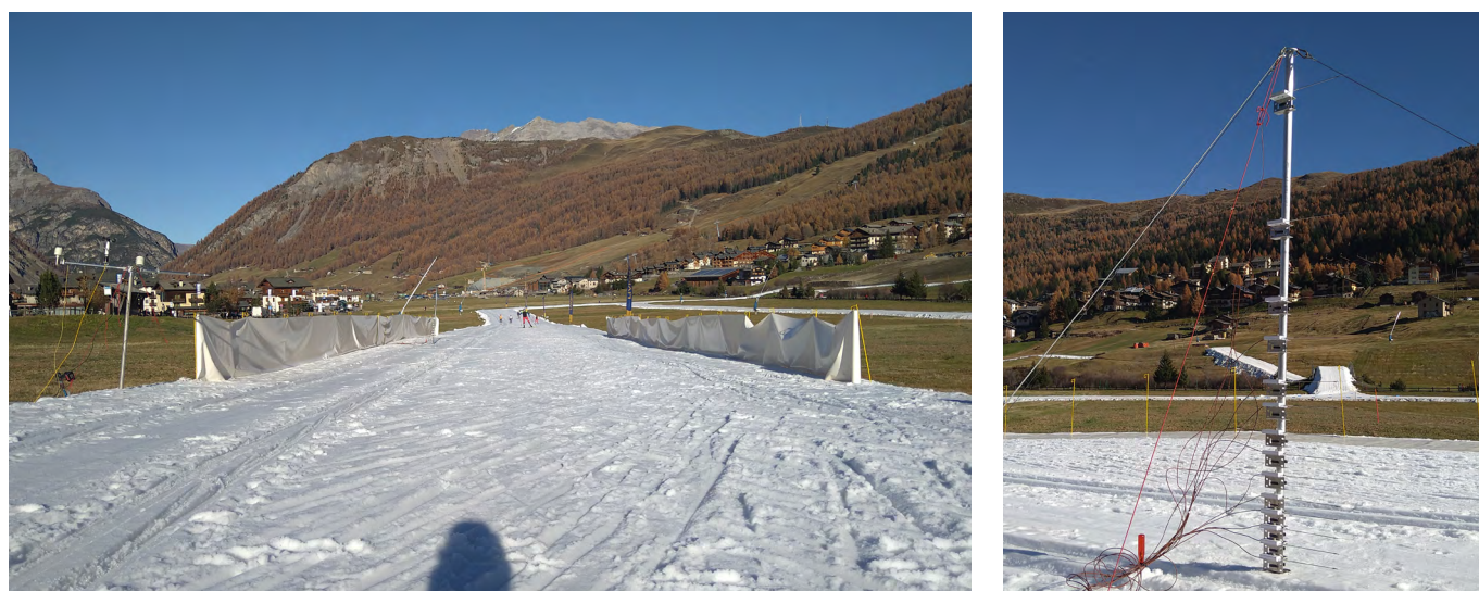
Figure 4 Experiments on the influences of wind fences on the turbulent heat flux from the air towards the snow. Left: Overview of the experimental setup at the cross-country track made of storage snow at Livigno, ITA (31 Oct. 2025) with mobile fences and a mobile weather station to measure air temperature and humidity, solar radiation and snow temperature. Right: Heat flux measurement station located in the middle of the fences with 15 sensors revealing differences of vertical air temperature profiles with and without fences.
